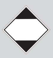
Limited quantities shipped by highway, rail, or vessel must display the limited quantity marking.
