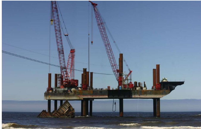
Barge with cranes held aloft on jacks.
