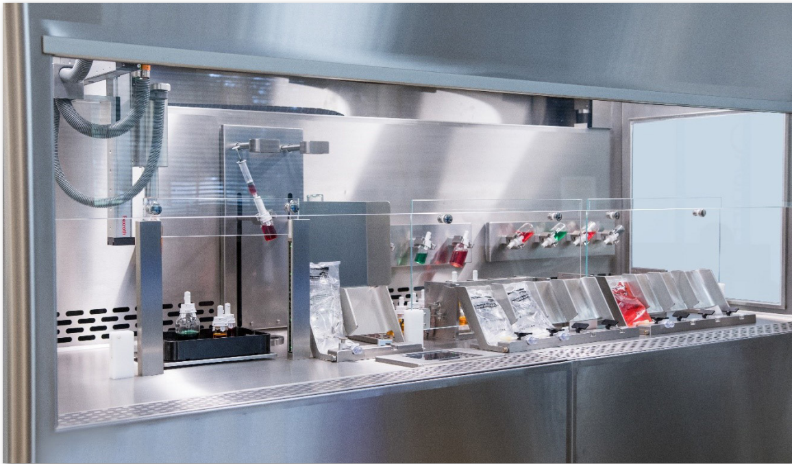
Figure 5. A robotic drug preparation system is considered a supplemental control.
